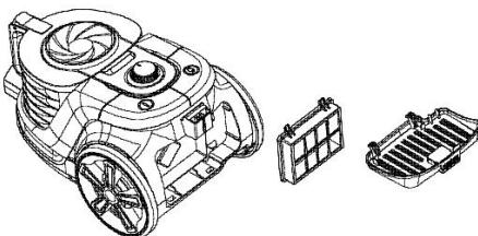
6. For rough cleaning, gently knock the dirt from the HEPA filter into the waste bin.
