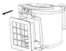
3. Press the latch to open the tray (1) and empty the dirt and dust.
